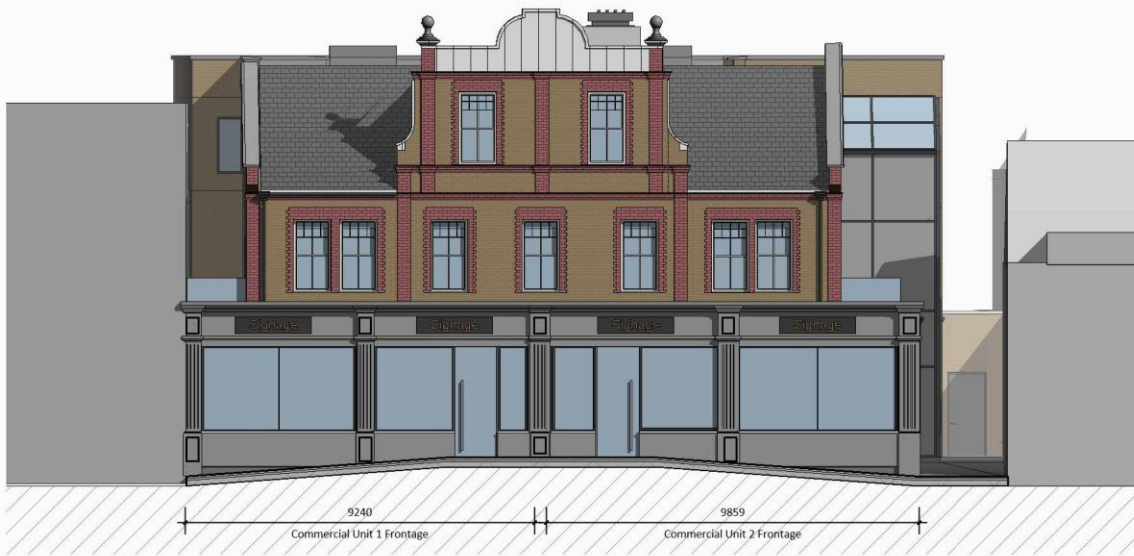
③ Commercial Units - Street Elevation 1 : 200
